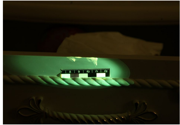
Fig. 1 Use 445nm laser to visualize traces of fine spots on white furniture
