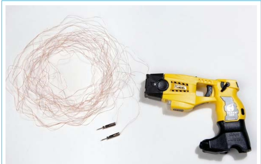
Figure 1. Taser® X26. The device propels two barbed darts connected to the gun by insulated conductors son, transmitting the electrical discharge (photo CEMCAV-CHUV)
