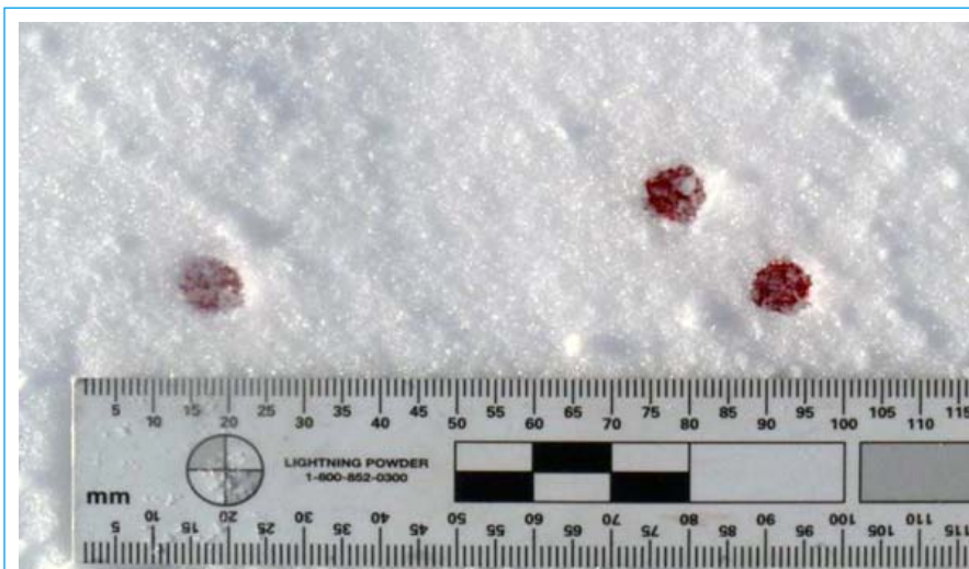
Figure 4. Drip stains from 100cm in soft snow resulting in a depression in the snow, reduced stain size (compared to 30cm drop height) and a near circular perimeter.
