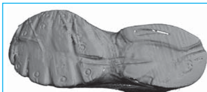
Fig. 3 A 3-D laser scanner image of the suspect shoe. Manipulation of the images in Figs 2 and 3 with an imaging software permits direct comparison and provides a demonstration tool for court purposes.
