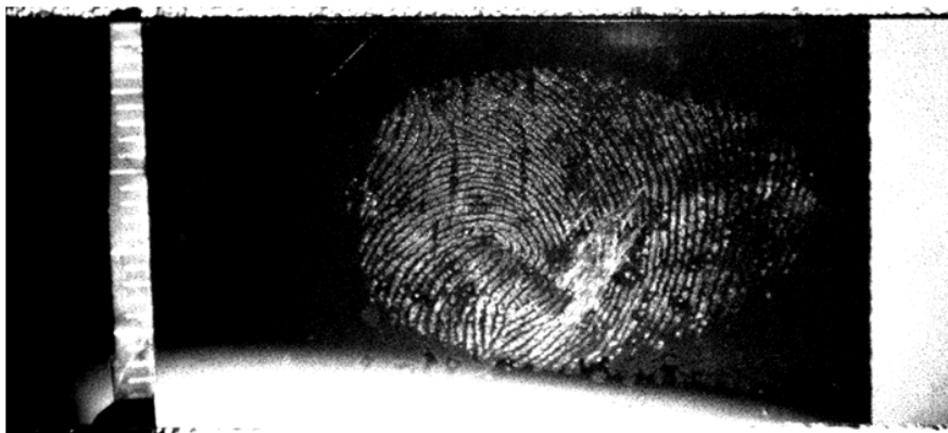
Fig.1 The sweat fingerprint on Glass Slide A got by using 254nm shortwave Ultraviolet reflectance imaging method. (Adjusted the luminance, contrast and gamma of the images to get the best showing effect)
