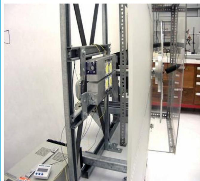
Fig. 12a LED array backlighting system on the adjustable Multistrut® frame, bolted to the MDF board.
