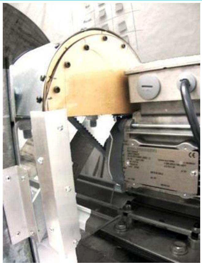
Fig. 11 The belt drive cover with the clear Perspex® walls.
