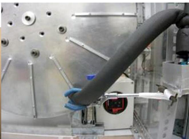
Fig. 7b The position of the insulated application hose and pump for upward-moving trials: 20 mm from the perimeter of the disc, 55 degrees from the horizontal, 15 mm from the surface of the disc and the pump (far right).
