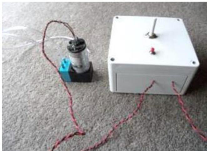
Fig. 6a KNF Neuberger® pump, rotary switch dial and activation button.
